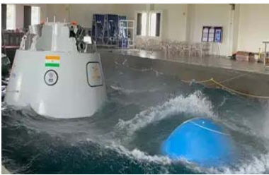
Figure-1 CMRM floating trials with sea state simulation
